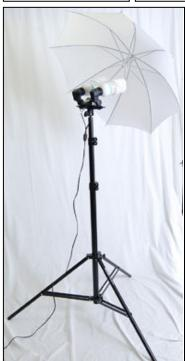
Once fully assembled, your continuous lighting kit should match that in Figure 11. To use, plug in the cord on the ac light socket and flip the power switch.
